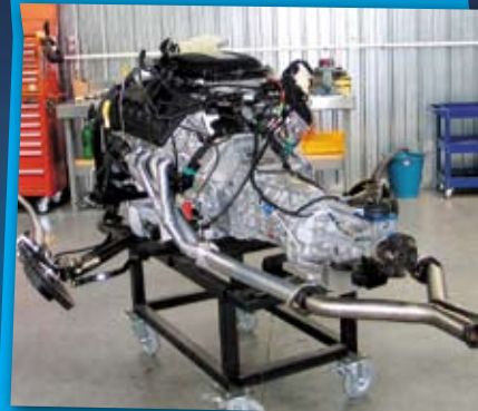
IPV ceramic-coated extractors, cat replacement pipes & 304 stainless steel X pipe Y section all fitted to engine and ready for installation
